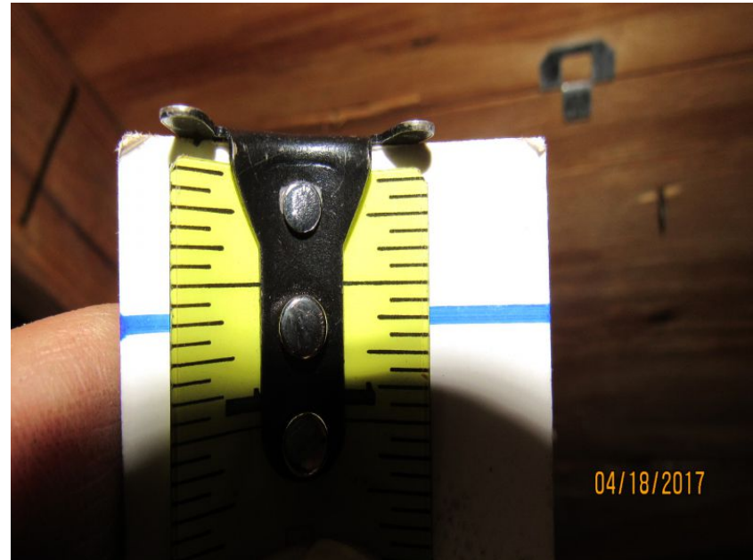
5/8" Deck Thickness Confirmed
